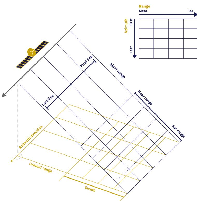
Figure 3.1 Definition of slant range and ground range
