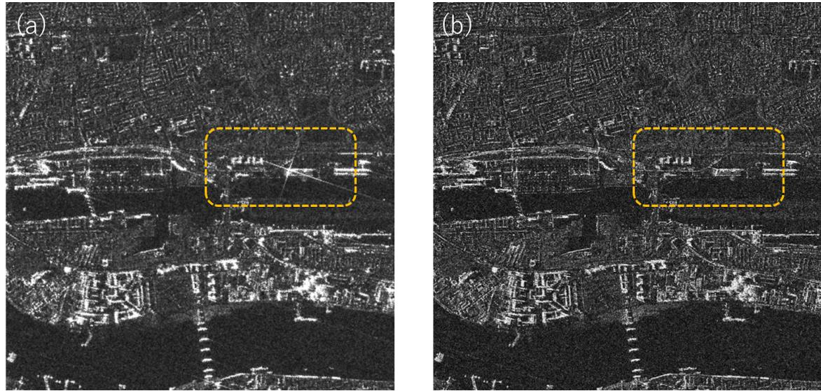
Figure 3.2 (a) 5m x 5m GRD image; (b) 1m x 1m SR-GRD image(Stripmap).
