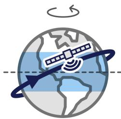
Figure 1.3 Inclined orbit
